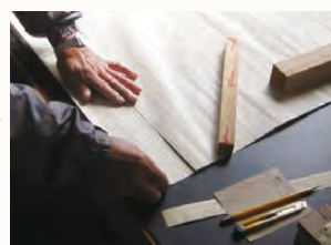
Welding veneer strips to make full size veneer sheets
